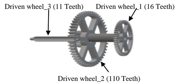
$$\text{Gear Ratio} = \frac{(\text{No. of teeth of Driven wheel}_3) 11}{(\text{No. of teeth of Driven wheel}_2) 110} = \frac{1}{10}$$
