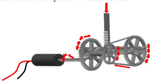
$$\text{Gear Ratio} = \frac{\text{No. of teeth of Driven wheel}}{\text{No. of teeth of Drive wheel}}$$
