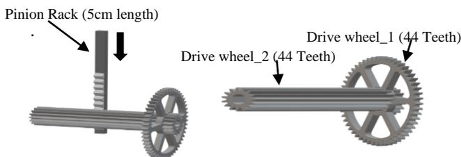
$$\text{Gear Ratio} = \frac{(\text{No. of teeth of Driven wheel}_1) 16}{(\text{No. of teeth of Drive wheel}_1) 44} = \frac{4}{11}$$
