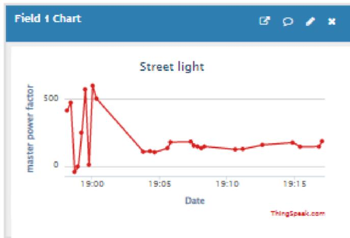
Fig. 13. Power consumption of master unit
