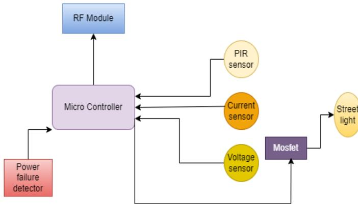
Fig. 3. Block diagram of the slave unit
